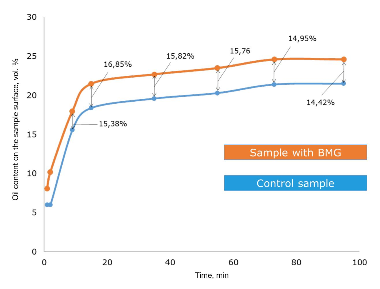
Oil level vs time curve, 3% BMG solution, Dosing 1 g/l
